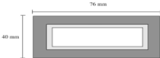
Plexiglass slide-form with a milling of 27 x 62 mm and a hole of 16 x 45 mm that will hold the coverslip of 24x60 mm
