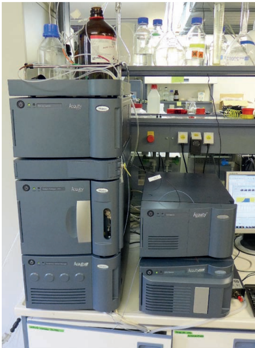
Figure 3 H-class UPLC system coupled to PDA-, FLR- and QDA-detector (Waters). Used for targeted analyses.
