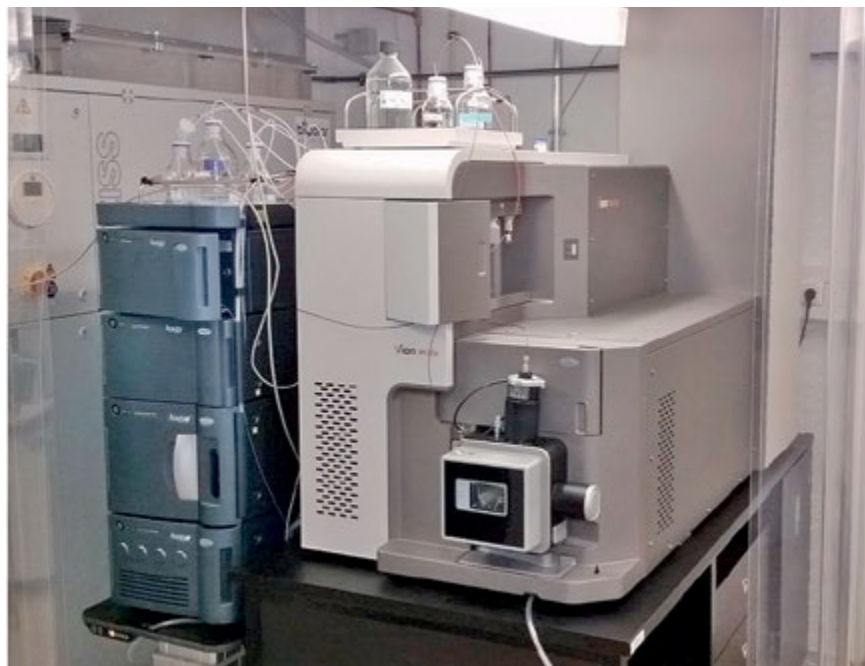
Figure 2 VION IMS-QToF MS system coupled to ACQUITY UPLC I-class system
